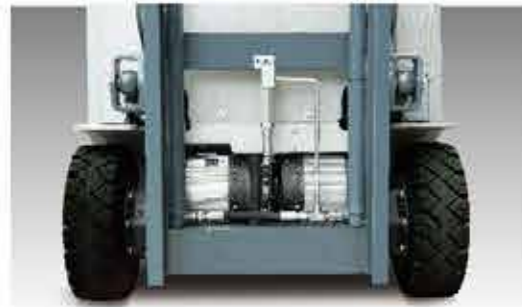
Front wheel dual drive motors provide more power.
