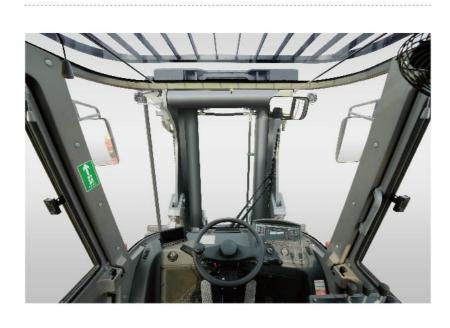
Excellent front view which is benefit for the work safety improvement and working efficiency is provide with high strength wide view mast and fork positioner with side shifting.
